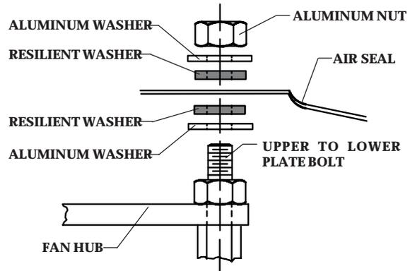
**AIR SEAL INSTALLATION ON AUTOMATIC HUB**
