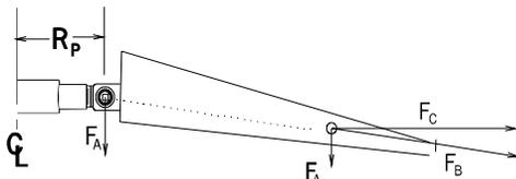
tions itself in the direction of this force with the result that the force is translated inward to the pivot point, as illustrated by the dotted line. The effect of this arrangement is exactly as if the total air load ( $F_A$ ) were applied at the pivot point rather than at the point outward on the blade. The maximum bending moment applied to the shaft by the air load is equal to the load ( $F_A$ ) multiplied by the distance from the fan centerline to the pivot point ( $R_p$ ).
