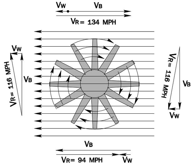
hour) with a horizontal component of wind velocity ( $V_w$ ) of 20 miles per hour. Note that the velocity ( $V_R$ ) of the fan blade relative to the air varies by a factor of 1.43. The blade load varies as the square of this velocity, or 2.05.
