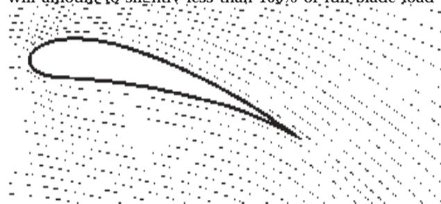
**AIRFLOW IN STALLING FLOW**
